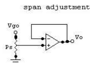
**Fig 2.6 Span Adjustment**
