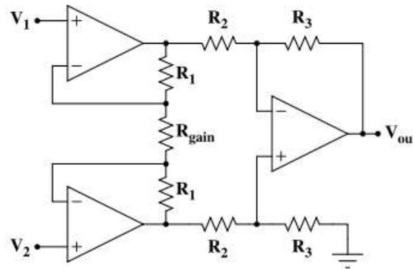
**Fig 2.4 The Most Commonly Used Instrumentation Amplifier Circuit is Shown In The Figure.**
