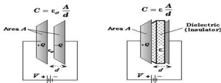
Fig. 2.3 Parallel Plate Capacitors
