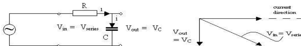
**Fig 2.5 Low Pass Filter**
