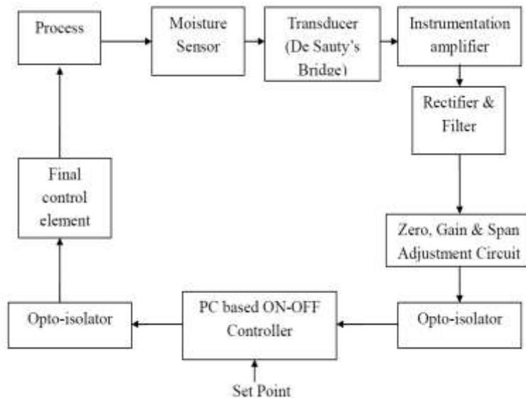
**Fig. 2.1 - Overall Block Diagram of The Proposed Project.**
