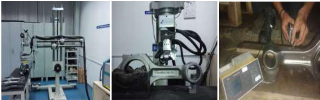
**Fig (2): X-stress analyzer (XRD); Measurement of residual compressive stress by XRD; Measurement of Surface roughness.**
