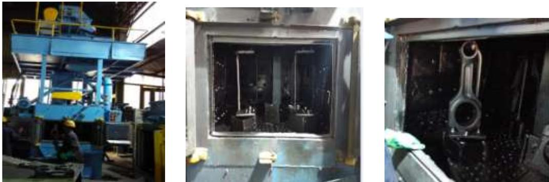
**Fig (1): Shows shot peening machine; Blasting Cabinet; Connecting rod mounted in cabinet**
