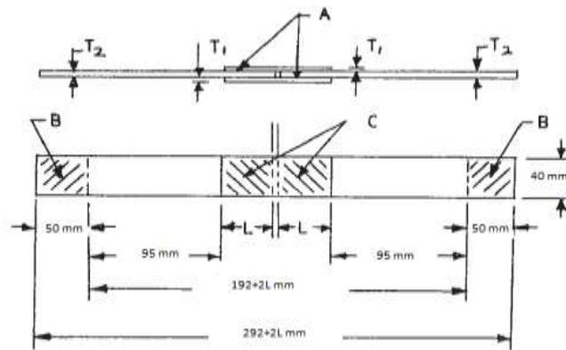
**Fig 8: ASTM Standard Double lap joint specimens with dimensions**
