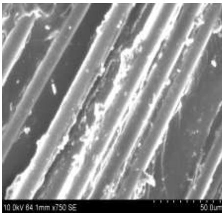
(a) Fiber Tear Failure
