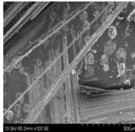
(b) Fiber Failure
