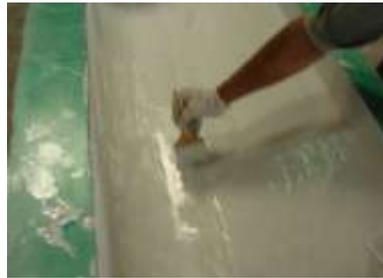
**Figure 4: Hand lay up process**
