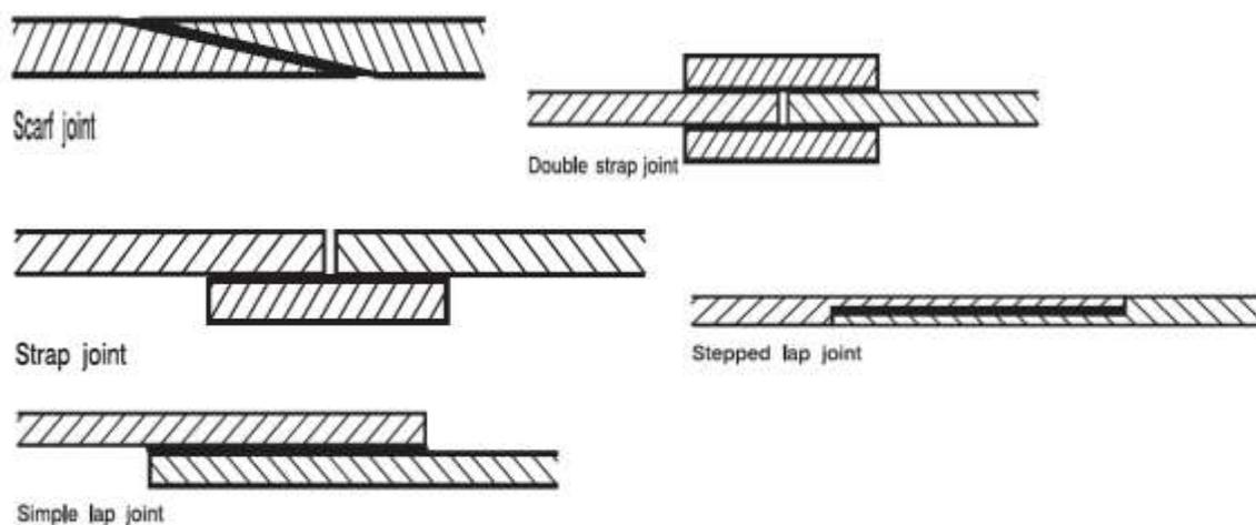
Fig 3: Types of joints.
