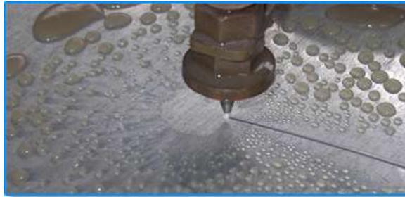
**Figure 6: Water jet cutting**
