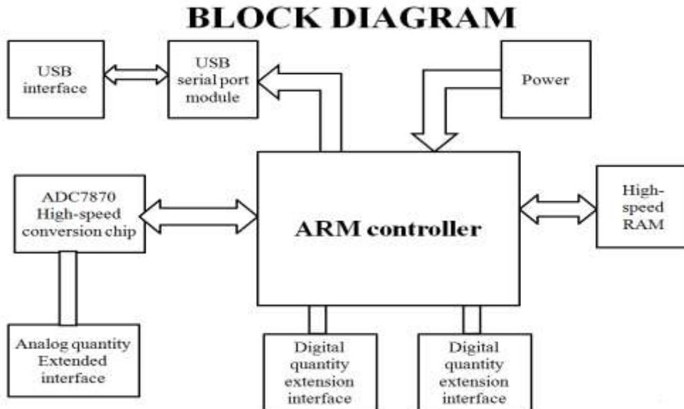
**Figure 1: Block Diagram of the Project**
