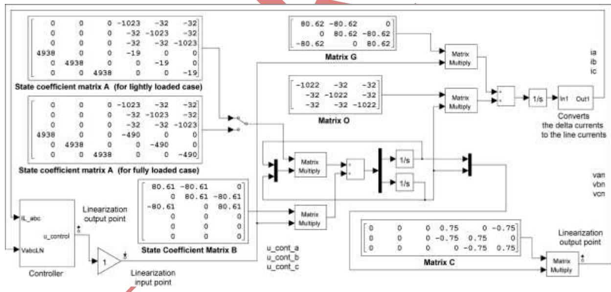
**Fig. 3. State-space model of the inverter power stage (the plant) including the closed-loop control system and the controller built in Simulink**
