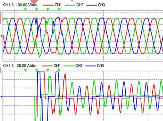
**Fig. 11. Measured three-phase output voltages and the load current of one phase for the following four cases**
