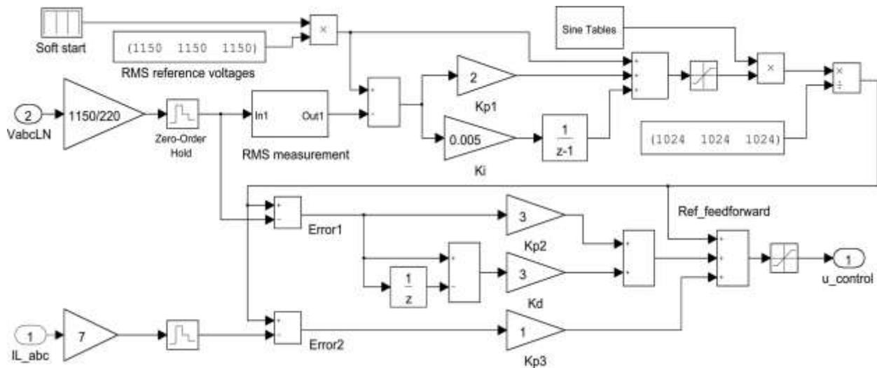
Fig. 4. Simulink model of the proposed multi loop controller
