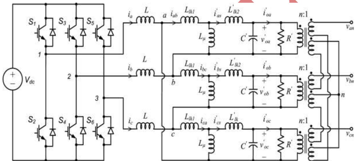
**Fig. 2. UPS inverter stage including the  $\Delta$ -zigzag transformer equivalent circuit and the resistive load**
