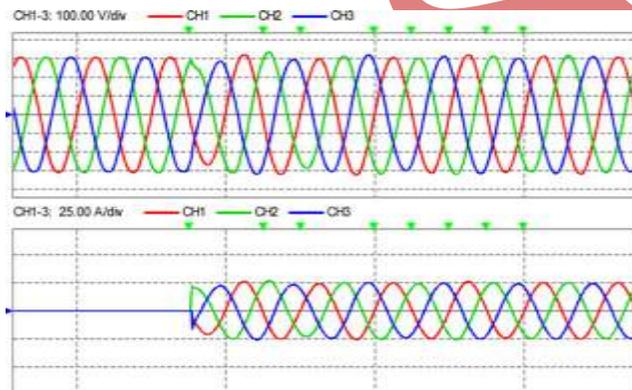
**Fig. 10. Measured transient response of output voltages (upper trace) and currents (lower trace)**
