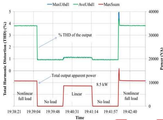
**Fig. 9. RMS fluctuations (top trace) and the profile of the percent THD of the output voltages (second trace) versus the load delivered by the inverter (bottom trace)**
