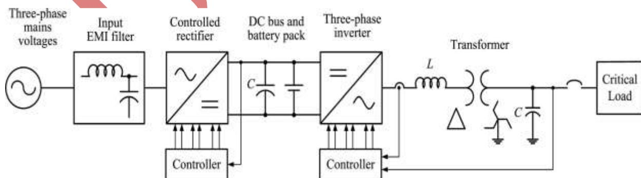
**Fig. 1. Single-line diagram of a typical three-phase four-wire transformer isolated UPS system**
