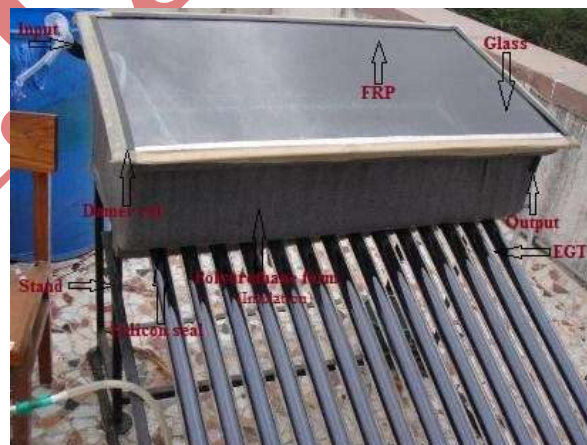
Fig.5. Solar still coupled with Evacuated glass Tubes
