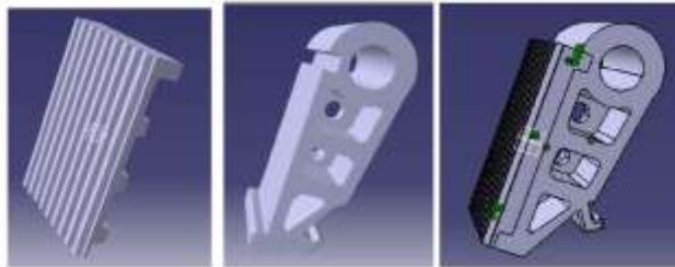
**Fig 5: Assembly of swinging jaw plate with pitman**
