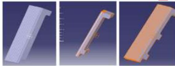
**Fig 4: Sketching of swinging jaw plate with one, two and three stiffeners**
