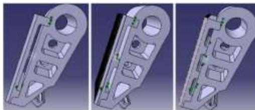
**Fig 6 swinging jaw plate with one stiffener, two stiffeners, three stiffeners**
