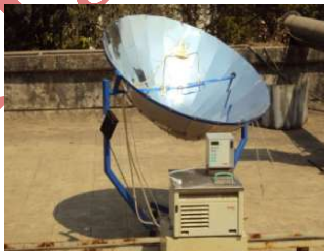
Figure 2: Experimental tup of photocatalytic degradation of meta-chlorophenolusing solar radiations.
