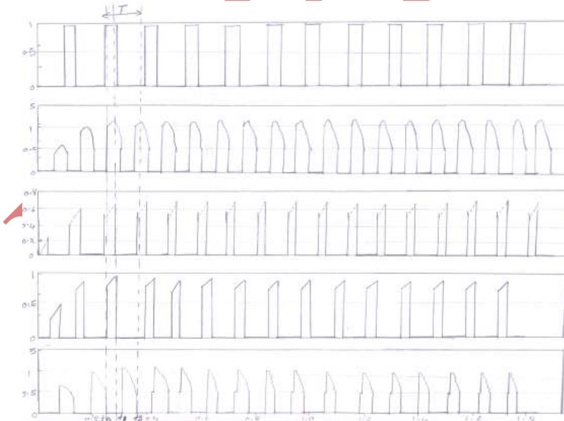
**Fig 2: Theoretical Waveform For CCM**
