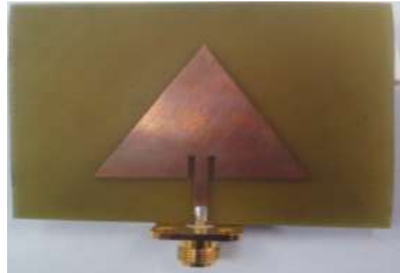
Fig.12 Fabricated Triangular Patch Antenna
