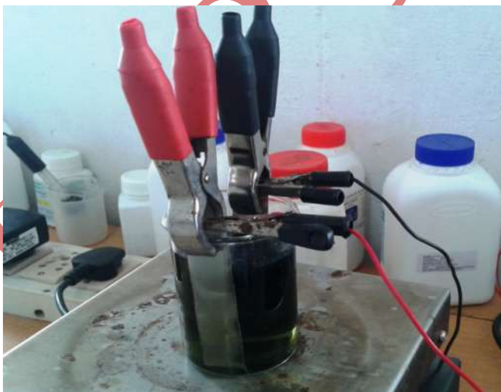
Figure 1: Experimental setup of electrodeposited Ni-Co-B thin films
