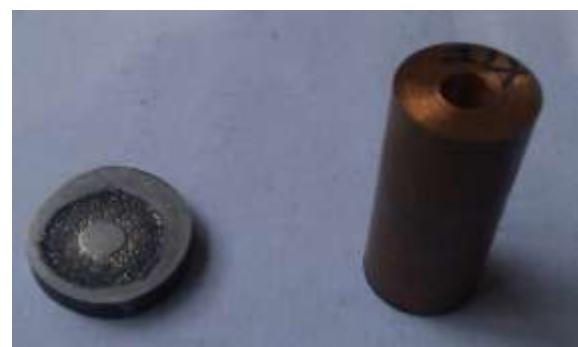
Fig. 4: Machining impression with Solid electrode and Tubular Electrode
