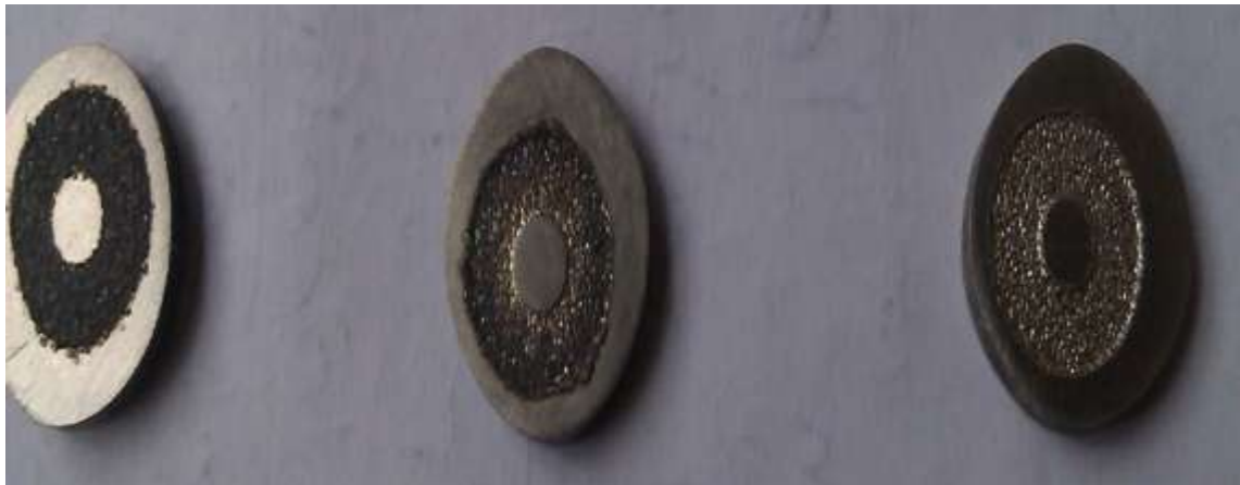
Fig. 5: Machining impression on Incoloy 800 ® by using dielectric as (a) oxygen (b) air and (c) kerosene
