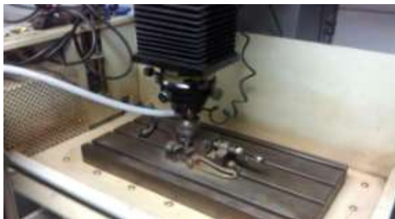
Fig. 2: Dry EDM setup for air as dielectric fluid
