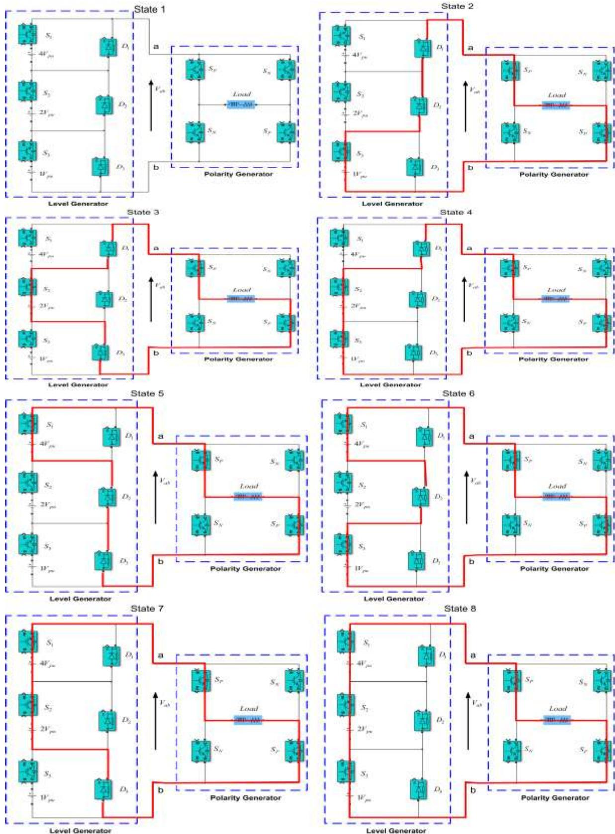
Fig 5: Operating States of the Proposed Inverter.
