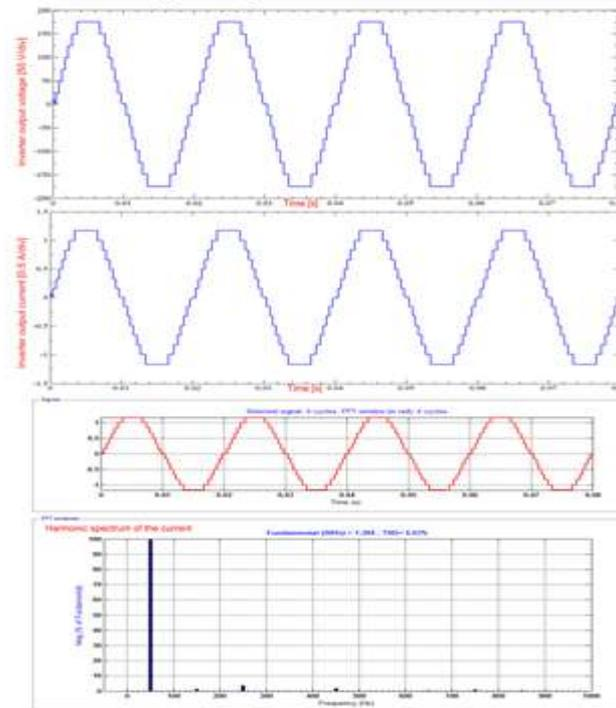
**Fig 6: Output waveform of the inverter feeding resistive load.**
