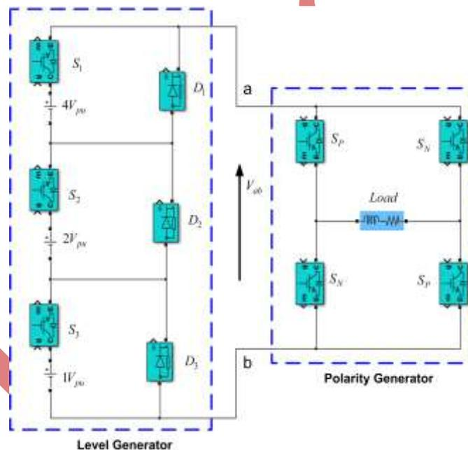
**Fig 1: Proposed Asymmetrical 15-Level Inverter Topology**
