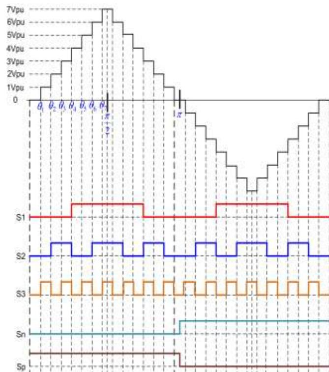
**Fig 2: Stepped-Voltage Waveform Consists of The Output Of Proposed Inverter Topology.**
