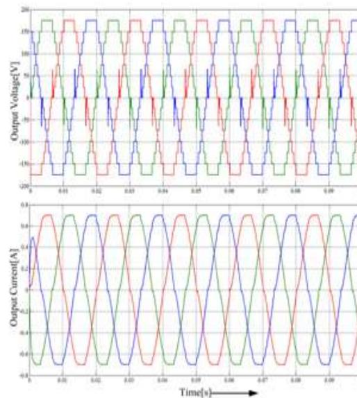
**Fig. 9. Output waveform of the proposed three phase inverter feeding resistive-inductive load**
