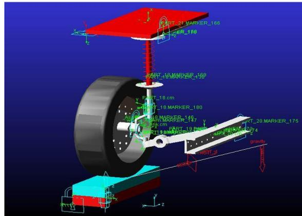
**Figure 2 Quarter Model of Existing Suspension System in ADAMS**
