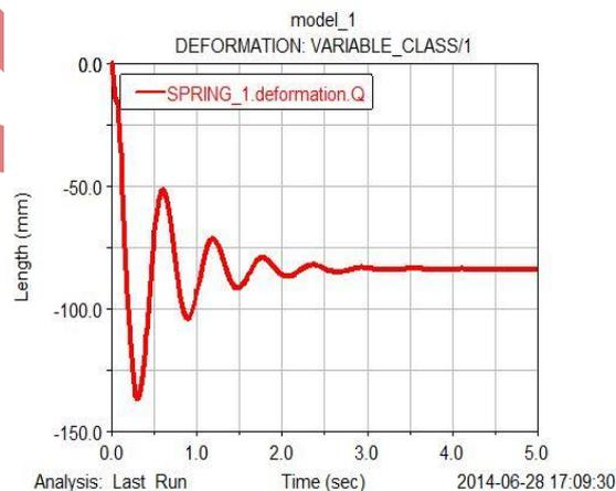
**Fig 3 Graph for Existing Suspension System with Kerb Weight**
