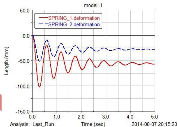
**Fig 5 Graph for Series Suspension System with Kerb**
