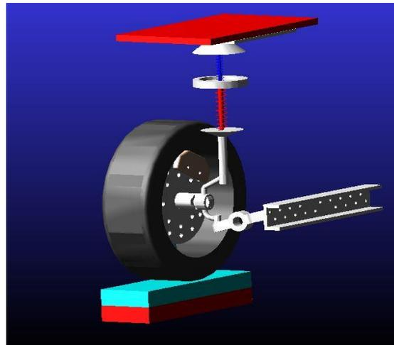
**Fig 4 Quarter Model of Modified Suspension System in ADAMS**
