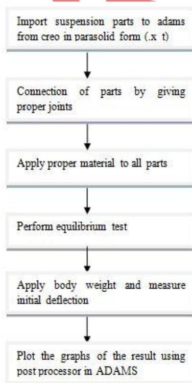
**Fig 1 Steps for Analysis Procedure in ADAMS**
