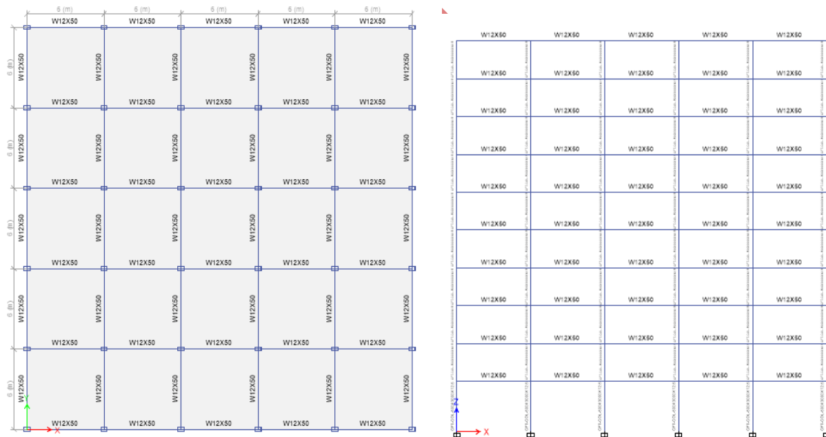
Fig 2. Plan and Elevation of ten-storied Composite (CFSRT column and Steel beam) moment resisting frame
