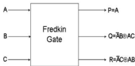
Figure 1: Fredkin Reversible Logic Gate
