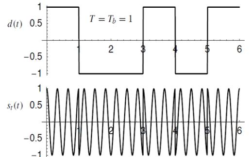
**Fig7. BPSK Using a Rectangle Pulse**
