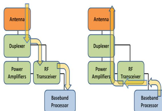
Figure 3. Block Diagram of Components of Mobile Systems
