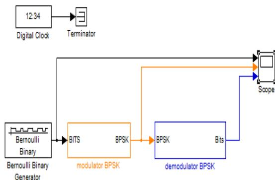
Figure 5. Simulink model of BPSK
