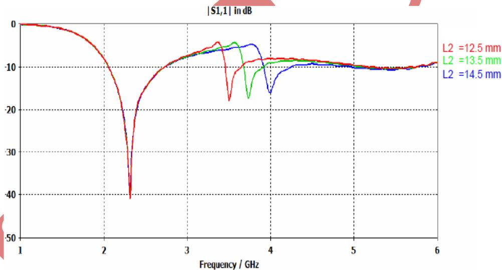
**Fig. 4 Simulated Return Loss of the radiating elements for various  $L_2$**
