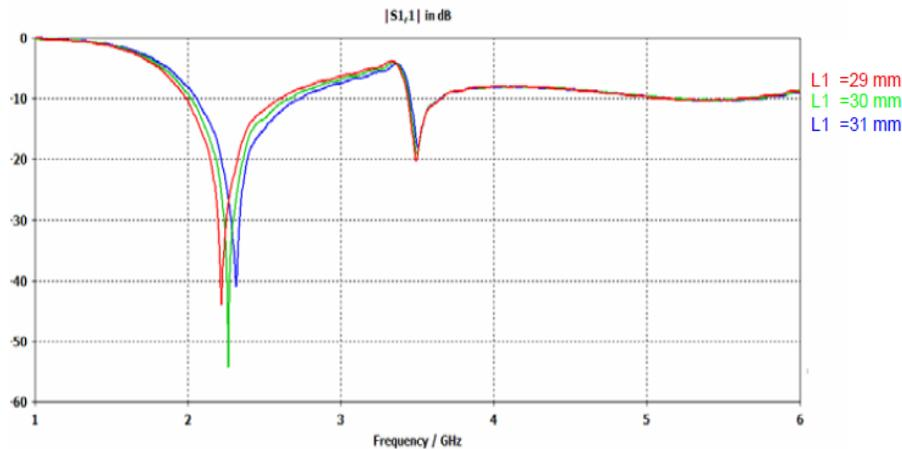
**Fig.3 Simulated Return Loss of proposed Antenna with various values of  $L_1$ .**
