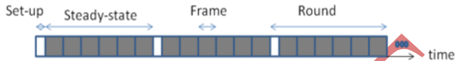
Fig 2: Time line showing LEACH operation. Adaptive clusters are formed during the set-up Phase and data transfers occur during the steady-state phase
