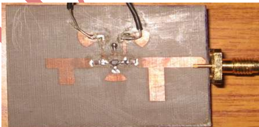
Fig. 4 Fabricated Circuit of the X-Band Oscillator
