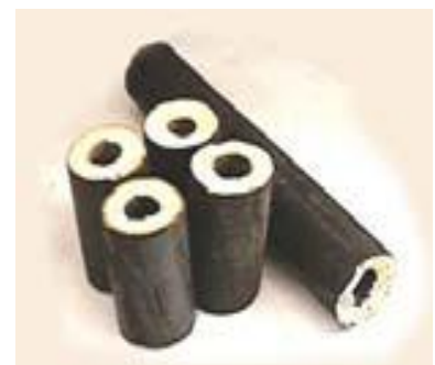
Fig. 6.2 Briquette made by screw extruder
