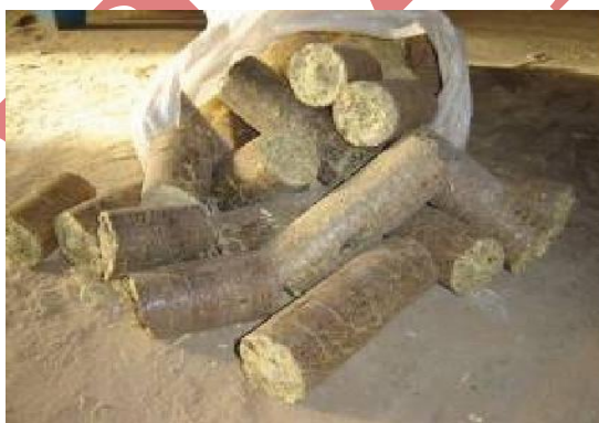
Fig. 6.1 Briquettes made from a hydraulic press
