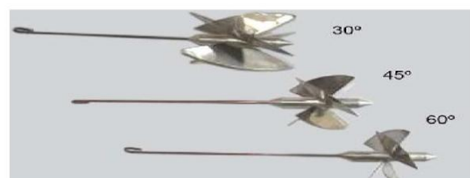
Fig3: Axial Guide Vane Swirler
