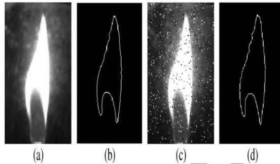
**Fig. 2.3 Example of noisy and processed flame images. (a) Original image.(b) Processed image of (a). (c) Original image with salt and pepper noise added.(d) Processed image of (c).**
