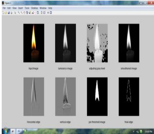
Fig 3.2 Flame Image Processing.
