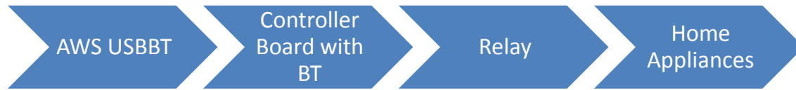
Fig 2: Working Principle of Application (Home Appliances Control System)
