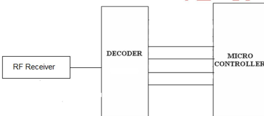
The received data at the transmitter receiver is decoded by the decoder IC (HT12D). The decoded data is used by the microcontroller for the further function.
