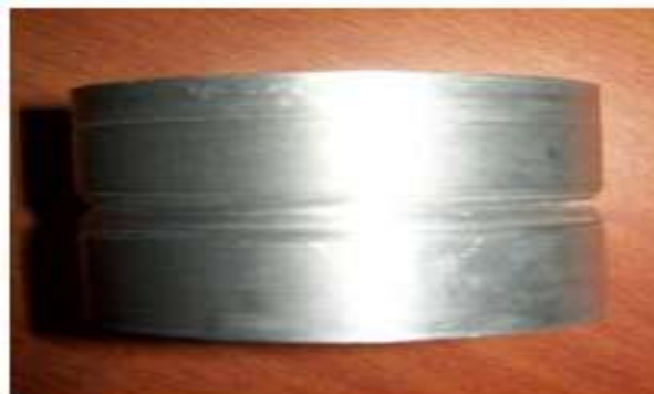
Fig. 5 Prepared Specimen of Center Intrude I
