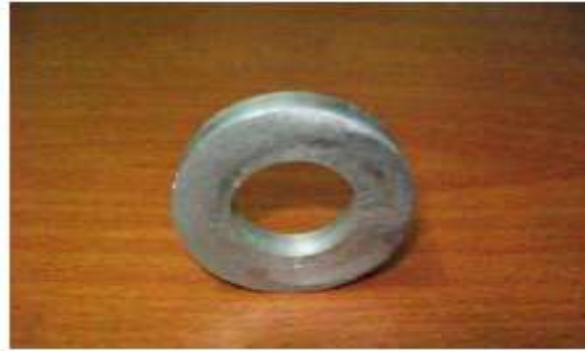
Fig.9 Deformed Ring Specimen Table 1: Specimens and FE Parameters
