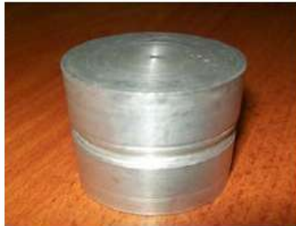
Fig. 5 Prepared Specimen of Center Intrude I
