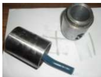
Fig. 1.6: Rod extrusion arrangement
