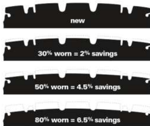
Fig. 2 Effect of Tread Depth on Fuel Consumption Fuel savings at various tread wear level [24]
