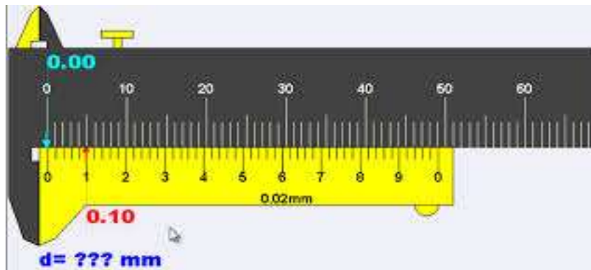
Figure 2: Typical Vernier Scale
