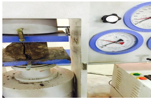
Fig.6- Split Tensile Strength Testing
