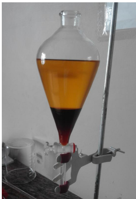
Fig.1. Separation of Mustard Methyl Ester and Glycerin
