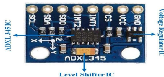
Fig. 2. ADLX345 hardware layout
