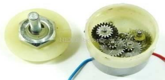
Fig. 1.4: 60 RPM Centre Shaft DC Motor
