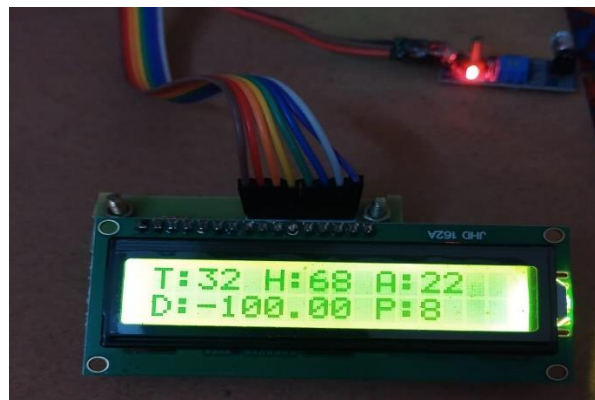
Fig. 10. Display of Ammonia, Humidity, Temperature on LCD.
