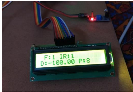
Fig. 10. Display of Water Flow, IR, PH, DO on LCD
