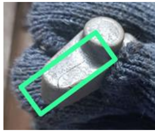
Figure 6: Crack Defect in Flange
