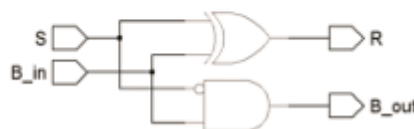
Figure 5.4: 1-bit subtractor with the input T = 0
