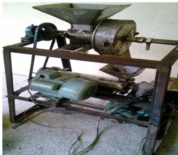
Fig 2. Motorized Ginger Juice Expression Machine [22].
