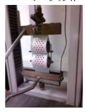
To sum up, our suggested approach is Measure the forces applied on the Geocell in your design. Verify the Geocell Geometry is retained for the entire design life
