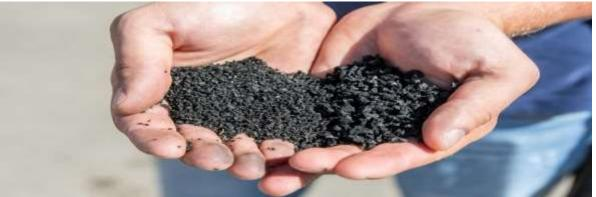
The use of waste tyres in construction of roads brings out a better performance. There is better binding of bitumen with waste tyres. The frequency of voids is also reduced due to increased bonding and area of contact between polyners and bitumen.
