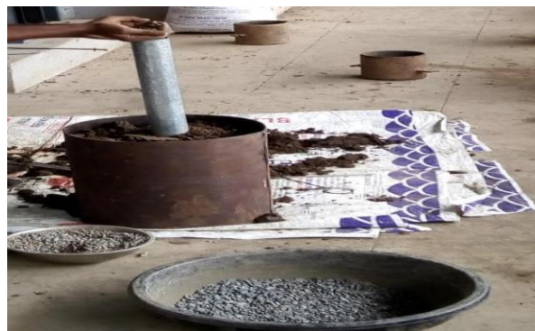
Fig 3.1 Experimental set-up showing compaction of soil and installation of GP
