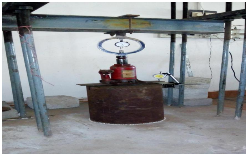
Fig 3.2 Pile Load test setup
