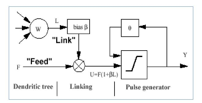
Figure 4. The block diagram of the pulse-coupled neuron
