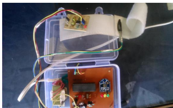
Fig.3 Temperature sensor transmitter
