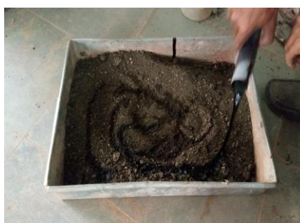
Fig.4.1: Black cotton soil with Bitumen emulsion
