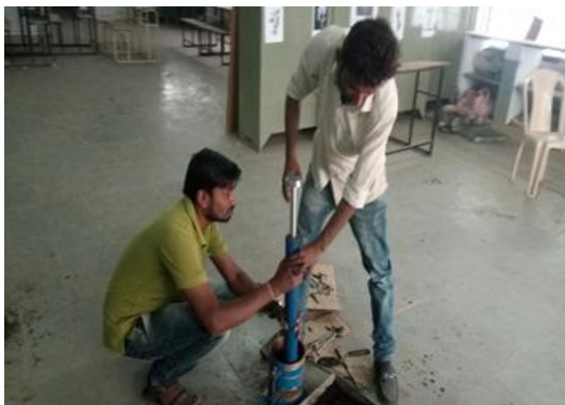
Fig.3 Preparation of CBR Mould
