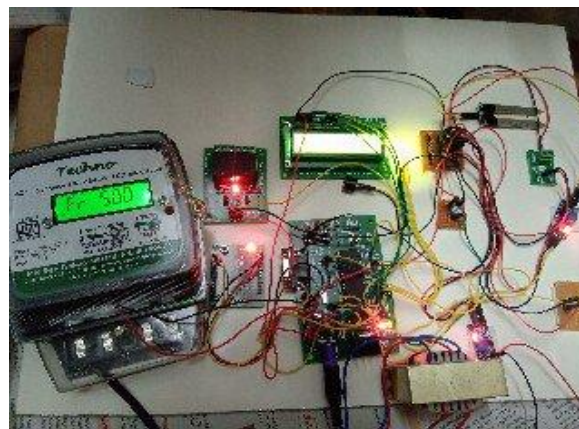
Fig4: prototype of transformer monitoring with prepaid energy meter
