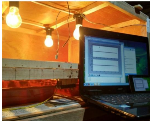
Figure1. Quail Egg Smart Incubator.
