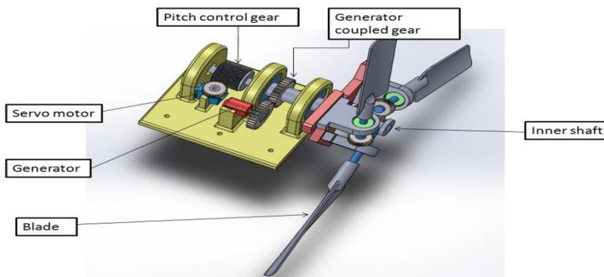
Fig 1.2:- Designed of wind turbine
