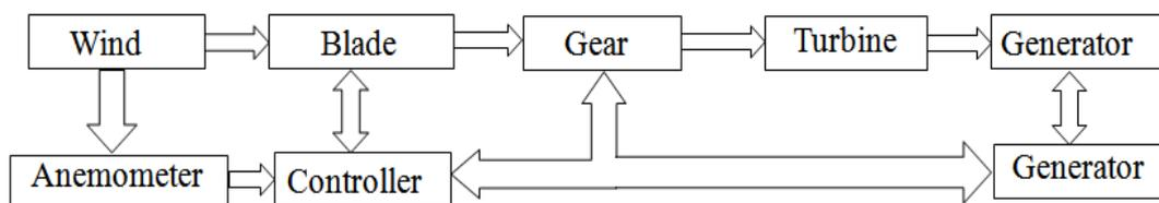
Fig 1.1:- Block Diagram
