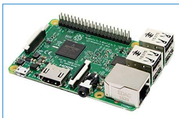
Fig: 2 RASPBERRY PI3 Processor for Detecting and Controlling Pollution
