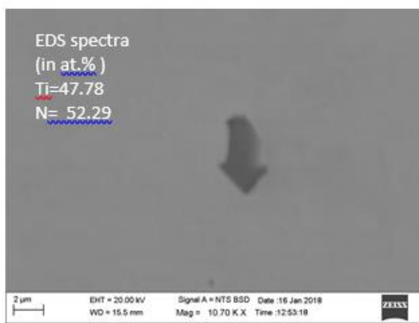
Fig. 11 SEM micrograph of the TiN inclusion and EDS analysis
