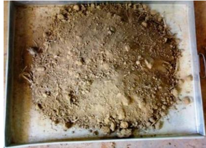
Fig 1 shows Poor graded sand collected at chainage of 1500m after digging to a depth of 300mm.
