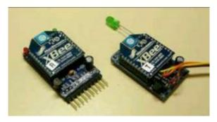
Fig.2.4 Zigbee Transmitter and Receiver
