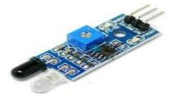
Fig.2.3 INFRARED SENSOR
